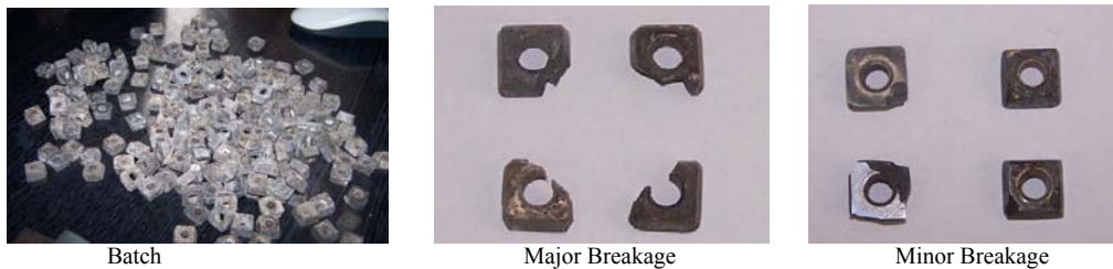
Figure 6. Major and Minor Breakage of the Tools
